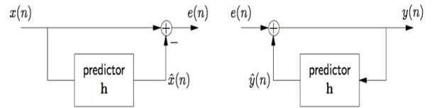
Fig 1. Subband adaptive open loop filtering
